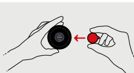
**Fix** the Magnetic Wall Mount on the back of the Airtame 2.
