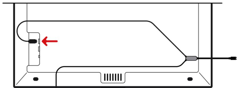
Plug in HDMI to the TV, and connect USB A to the power supply. **Always use** the provided power supply to power the Airtame 2.
